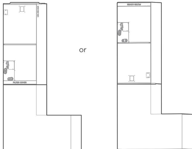
**Fixing instructions:** When installed vertically (upward or downward), the lower end of the air outlet needs to be connected to the L-shaped metal air duct and fastened by screws
