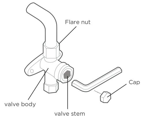
13. Using hexagonal wrench, fully open both the high pressure and low pressure valves.
