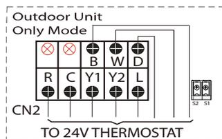
24V must never be connected to S1 - S2. All wiring must be in compliance with the above scenarios. Incorrect wiring will cause irreversible damage to control.
