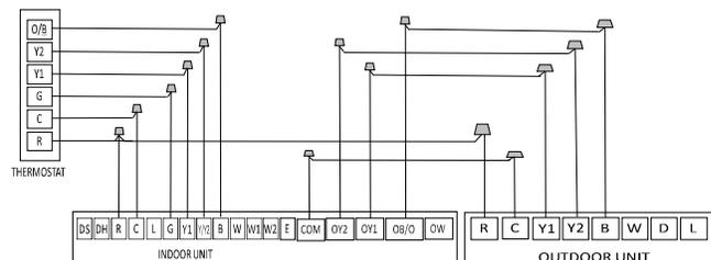
• Wiring for 3H and 2C thermostat
