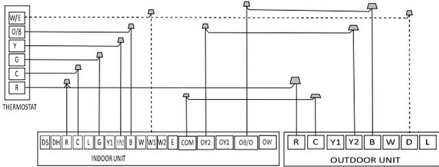
S4-4 Default on, W1 and W2 shorted for single stage Aux heat operation. Turn off to separate stages.
