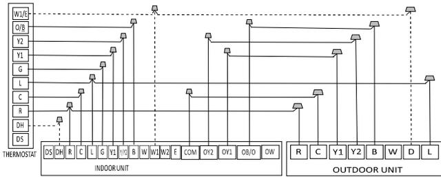
S4-2 Default on, DH function off. Turn switch off to activate DH function.
