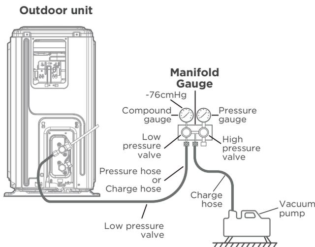
6. Run the vacuum for at least 15 minutes, or until the Compound Meter reads  $-76\text{cmHg}(-10^5\text{Pa})$  or 500 microns.
